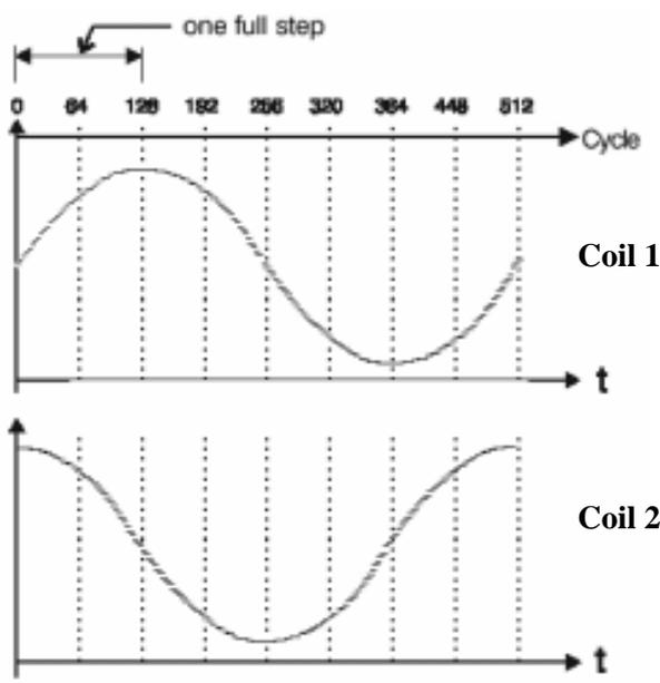
The basic principle is to produce, according to an 8-bit range of 0-255, two currents 90 out-of-phase with each other, for the two phases of the motor. This is as though each motor is controlled by a two-channel current amplifier, where each current value is represented by an 8-bit value. The motor is supplied with the correct values of phase current by the transmission of the 8-bit values to two defined port addresses.
