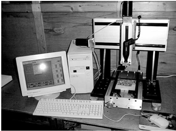
Fig.5. The general view of developed system (controller + CNC machine)
