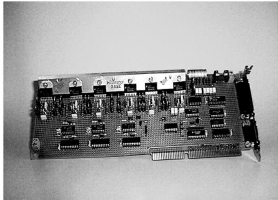
Fig.6. The general view of microstepping control card.
