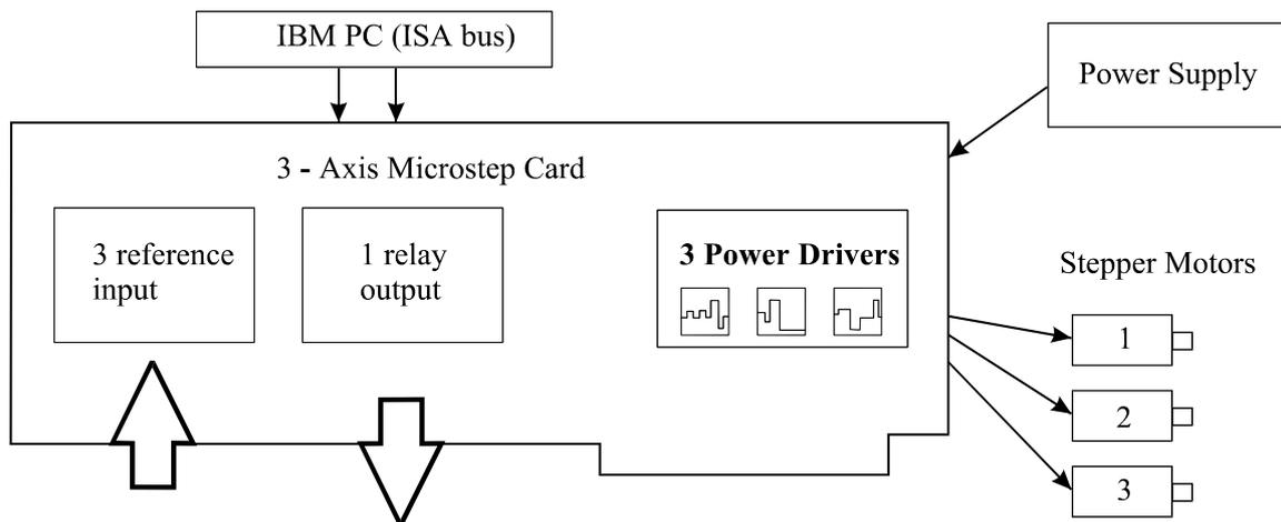
Fig.1. The block scheme of microstepping card.
